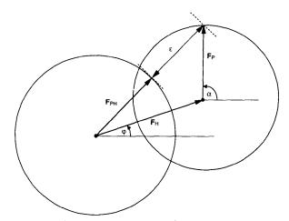
Fig. 1. Relation between the structure-factor amplitudes of native molecule ( $\mathbf{F}_{P}$ ), substituting atoms ( $\mathbf{F}_{H}$ ), and the substituted compound ( $\mathbf{F}_{PH}$ ). Lack of closure ( $\varepsilon$ ) defines the difference between the magnitudes of calculated  $\mathbf{F}_{PH}$  and observed  $\mathbf{F}_{PH}$ .
