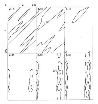
Fig. 6. Contour maps of a cross rotation function as produced by the program written by Crowther (1972) and modified by Dodson (1985). GP1 and GP2 denote the true positions. The contour levels are 60 and 80% of the maximum value of the function.
