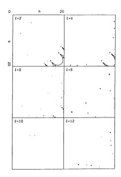
Fig. 5. Percentage errors of  $T^{i}(h, k)$  when evaluated by means of a 12-point Legendre-Gauss integration formula, with  $h_{max}$  the same as in Fig. 2. The contour levels are now 0.1 and 1%.
